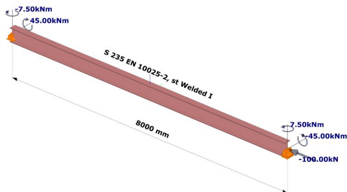
Fig.45 Simple fork supported member with IPE360 section subjected to biaxial bending and compression
